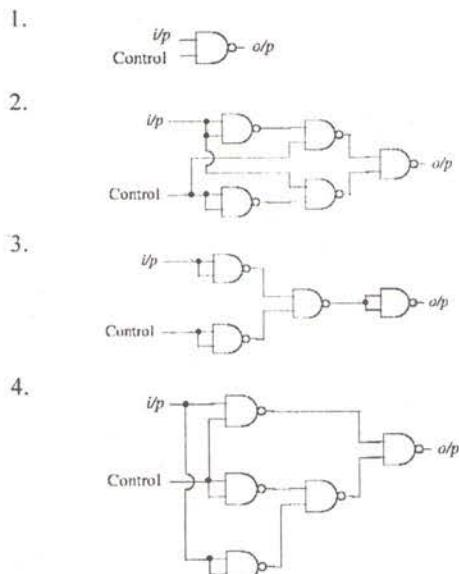
40. Which of the following circuits behaves as a controlled inverter?
